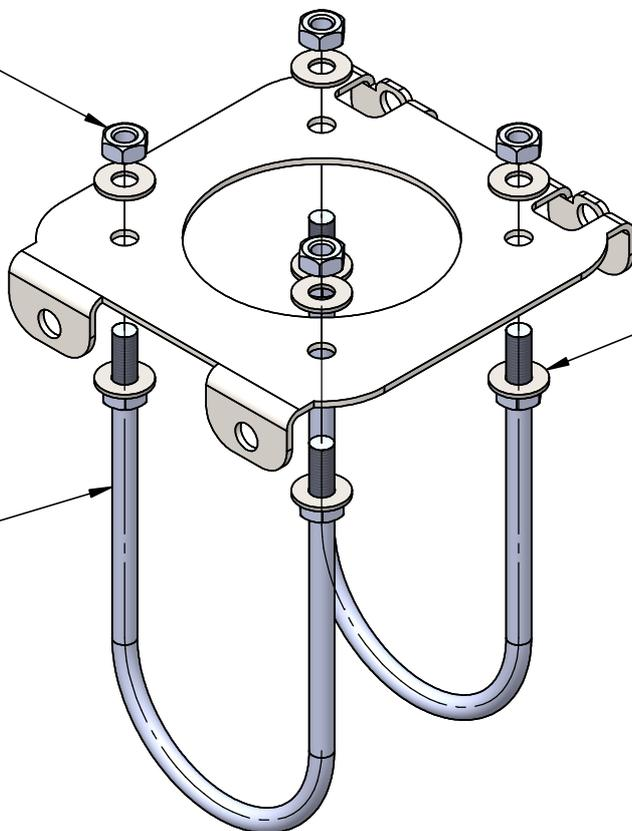
③ Ensure nuts and washers are wound to the bottom of the U-bolt threads
